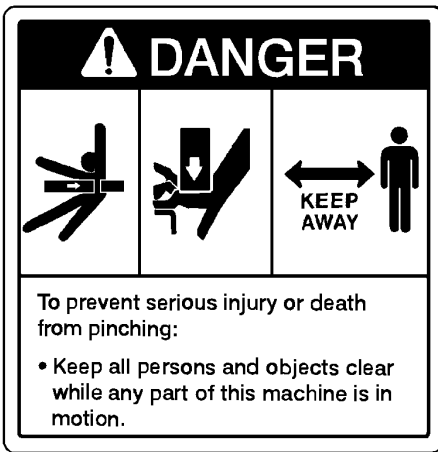
PART #40149 DANGER! PINCH POINT
