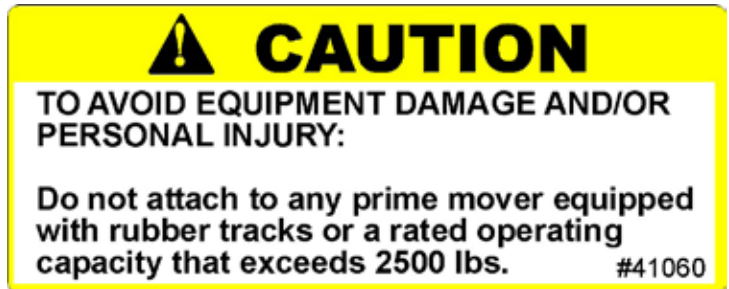
PART #41060 CAUTION! OPERATING LIMITATIONS
